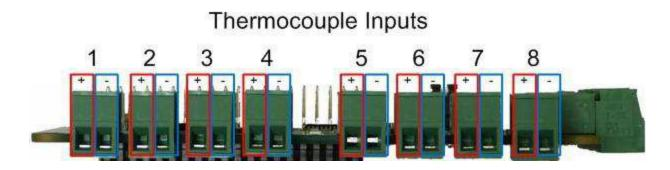
Each input has a plus and minus terminal. The guide below shows the common markings for type K and type J thermocouples:
