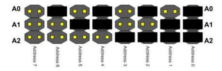
Starting with the THERMOplate, it is now possible to change the address of the board without having to perform a power cycle.
