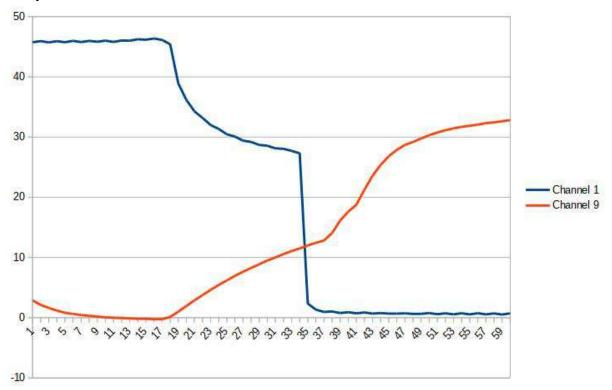
We started with the channel 9 sensor in an ice water bath and the channel 1 sensor jammed into an LED desk lamp. Then we let each sensor go back to room temperature for a couple of minutes. Finally, we swapped the position. It's apparent that the thermocouple responds much faster to temperature changes than the DS18B20.
