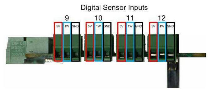
The DS18B20 can be purchased as a discrete component or preassembled with wires and a protective tip. Pi-Plates sells the latter with 1 meter cables. In most cases the wires are colored red for 5V, black for Ground, and blue or yellow for the digital signal. Here is a picture of one of our cables connected to the terminal block plug:
